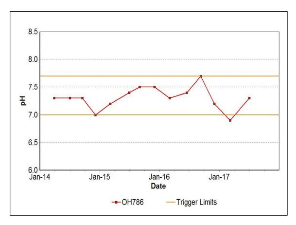
Figure 47: Hunter River Alluvium 1 Seam pH Trend - June 2017
