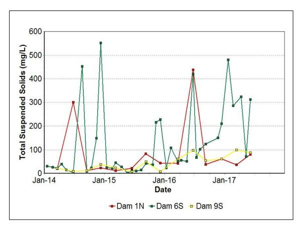
Figure 11: Site Dams Total Suspended Solids Trend 2014 – Current
