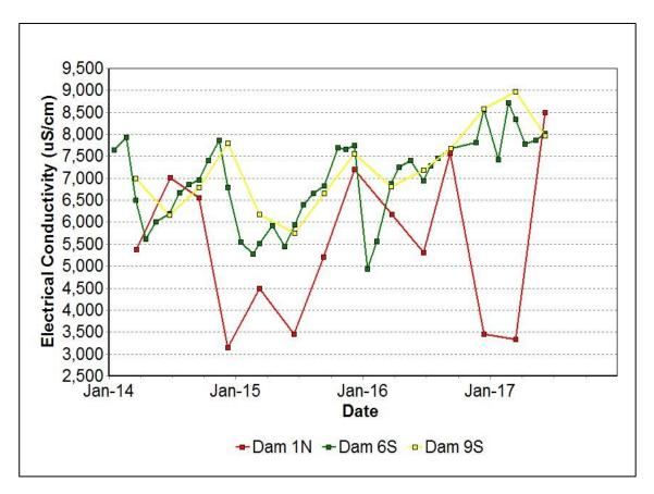
Figure 9: Site Dams Electrical Conductivity Trend 2014 – Current
