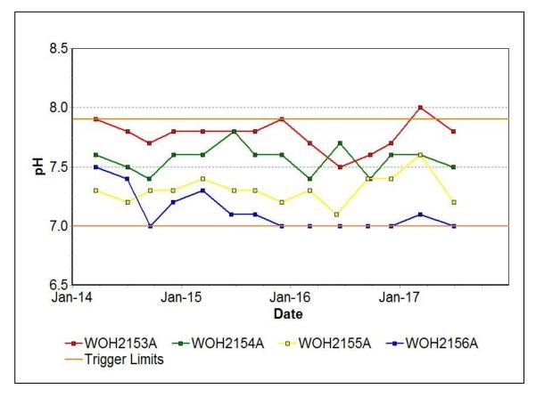
Figure 26: Redbank Seam pH Trend – June 2017
