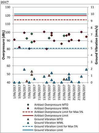
Figure 61: Bulga Village Blast Monitoring Results – June 2017
