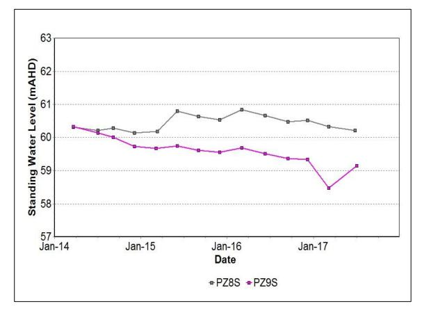
Figure 42: Wollombi Alluvium Standing Water Level Trend - June 2017
