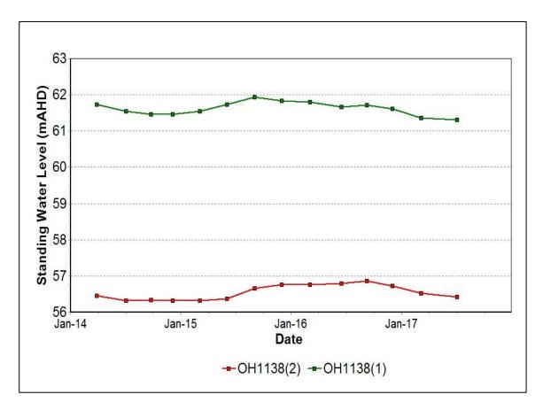
Figure 39: Warkworth Seam Standing Water Level Trend - June 2017
