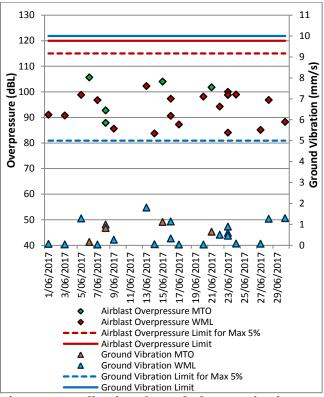
Figure 65: Wollemi Peak Road Blast Monitoring Results - June 2017
