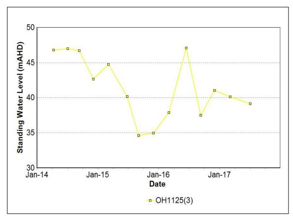
Figure 24: Bowfield Seam Standing Water Level Trend - June 2017
