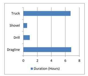
Figure 68: Operational Downtime by Equipment Type – June 2017
