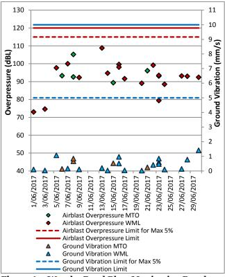
Figure 64: Wambo Road Blast Monitoring Results – June 2017
