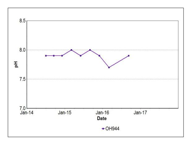
Figure 55: Hunter River Alluvium 5 Seam pH Trend - June 2017
