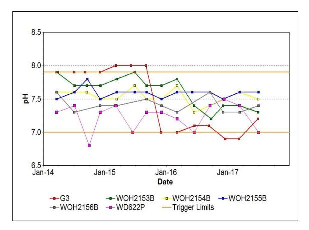
Figure 35: Wambo Seam pH Trend – June 2017
