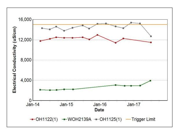
Figure 19: Blakefield Seam Electrical Conductivity Trend - June 2017
