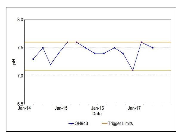
Figure 53: Hunter River Alluvium 4 Seam pH Trend - June 2017
