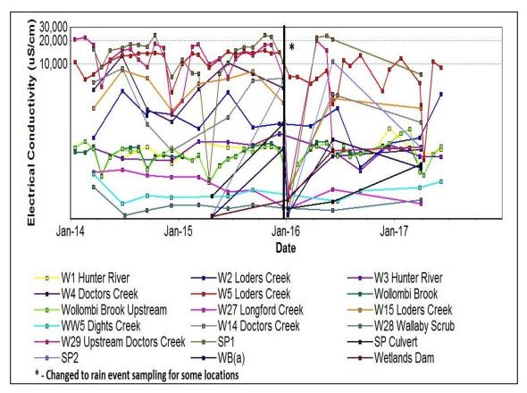
Figure 12: Watercourse Electrical Conductivity Trend 2014 - Current
