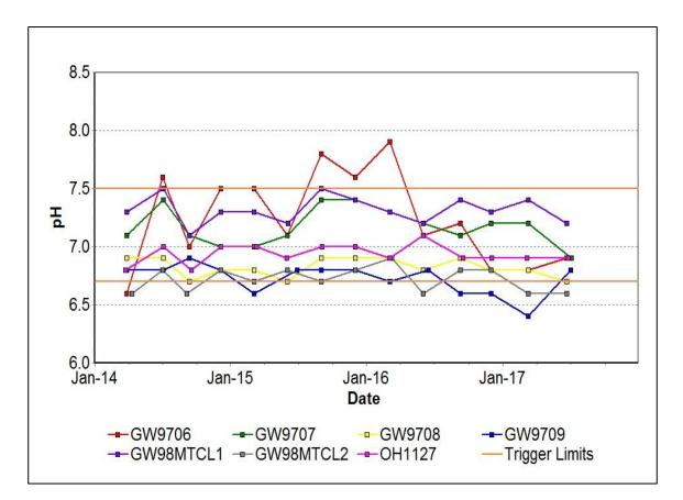
Figure 17: Bayswater Seam pH Trend June 2017
