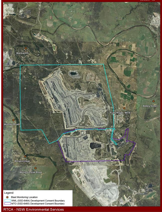
Figure 66: Blast and Vibration Monitoring Location Plan
