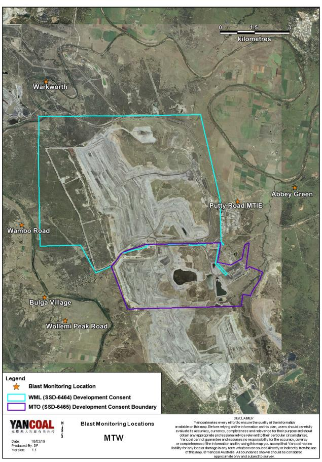
Figure 69: Blast and Vibration Monitoring Location Plan
