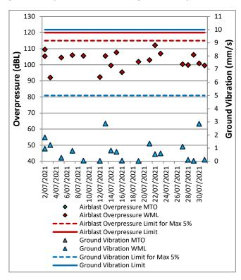
Figure 10: Bulga Village Blast Monitoring Results – July 2021
