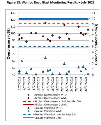
130 11 10 120 Ground Vibration (mm/s) 110 Overpressure (dBL 100 90 80 70 3 60 2 50 1 12/07/2021 22/07/2021 26/07/2021 28/07/2021 6/07/2021 10/07/2021 14/07/2021 16/07/2021 18/07/2021 20/07/2021 24/07/2021 30/07/2021 8/07/2021 Airblast Overpressure MTO Airblast Overpressure WML Airblast Overpressure Limit for Max 5% Airblast Overpressure Limit Ground Vibration MTO Ground Vibration WML Ground Vibration Limit for Max 5% Ground Vibration Limit
