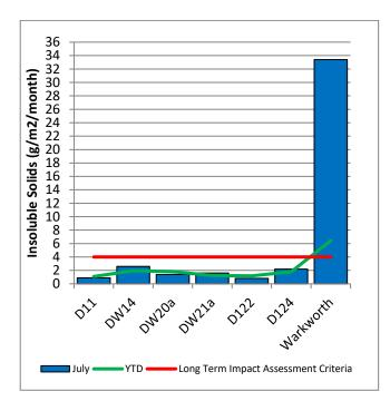
Figure 4: Depositional Dust – July 2021
