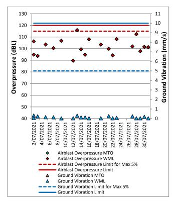
130 11 120 Ground Vibration (mm/s) 110 8 100 Overpressure ( 90 80 4 70 3 60 2 50 1 40 28/07/2021 4/07/2021 20/07/2021 22/07/2021 26/07/2021 2/07/2021 6/07/2021 8/07/2021 12/07/2021 14/07/2021 16/07/2021 18/07/2021 24/07/2021 Airblast Overpressure MTO Airblast Overpressure WML Airblast Overpressure Limit for Max 5% Airblast Overpressure Limit Ground Vibration MTO Ground Vibration WML Ground Vibration Limit for Max 5% Ground Vibration Limit
