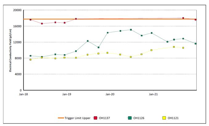
Figure 32: Vaux Seam Electrical Conductivity Trend – December 2021
