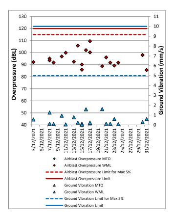
Figure 71: Wambo Road Blast Monitoring Results – December 2021
