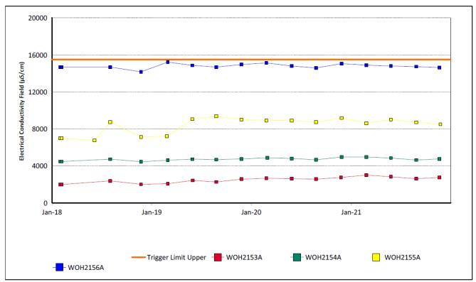
Figure 26: Redbank Seam Electrical Conductivity Trend – December 2021
