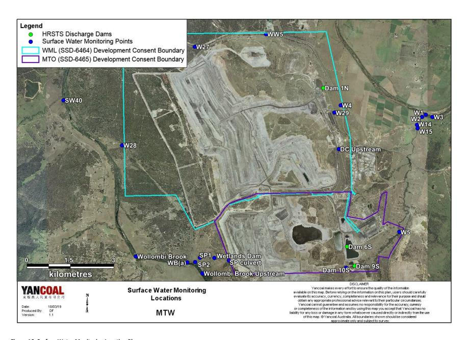
Figure 16: Surface Water Monitoring Location Plan
