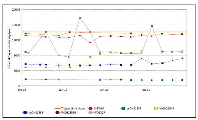
Figure 35: Wambo Seam Electrical Conductivity Trend – December 2021
