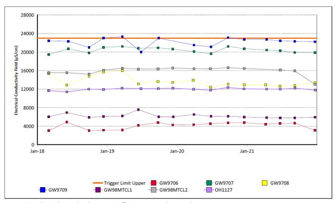
Figure 17: Bayswater Seam Electrical Conductivity Trend – December 2021
