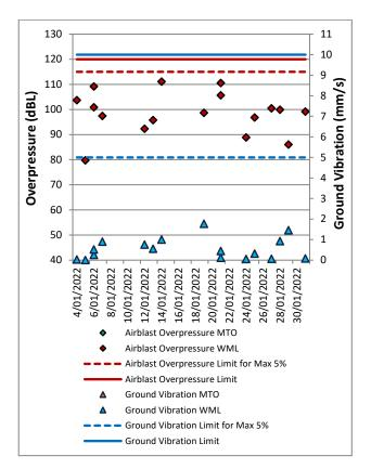
Figure 12: Wollemi Peak Road Blast Monitoring Results – January Figure 14: Warkworth Blast Monitoring Results – January 2022 2022
