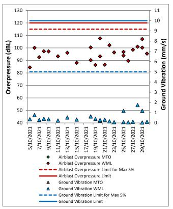
Figure 12: Wollemi Peak Road Blast Monitoring Results – October Figure 14: Warkworth Blast Monitoring Results – October 2021
