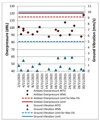
Figure 13: Wambo Road Blast Monitoring Results - November 2021
