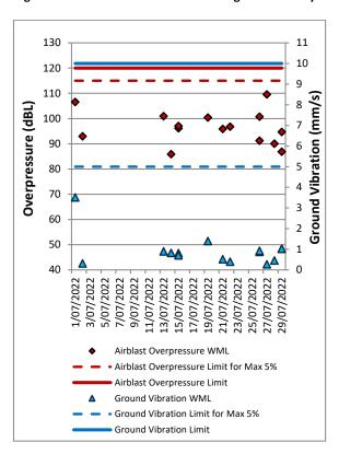
Figure 14: Warkworth Blast Monitoring Results – July 2022
