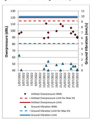
Figure 12: Wollemi Peak Road Blast Monitoring Results – July 2022
