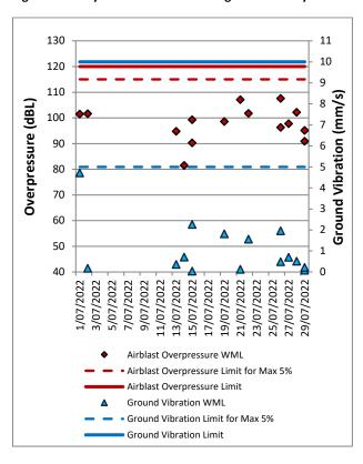
Figure 10: Bulga Village Blast Monitoring Results - July 2022
