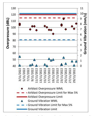
Figure 13: Wambo Road Blast Monitoring Results – November 2022
