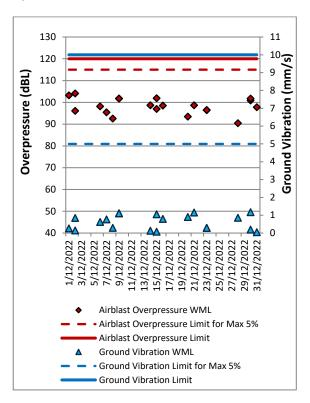
Figure 69: Wambo Road Blast Monitoring Results - December 2022
