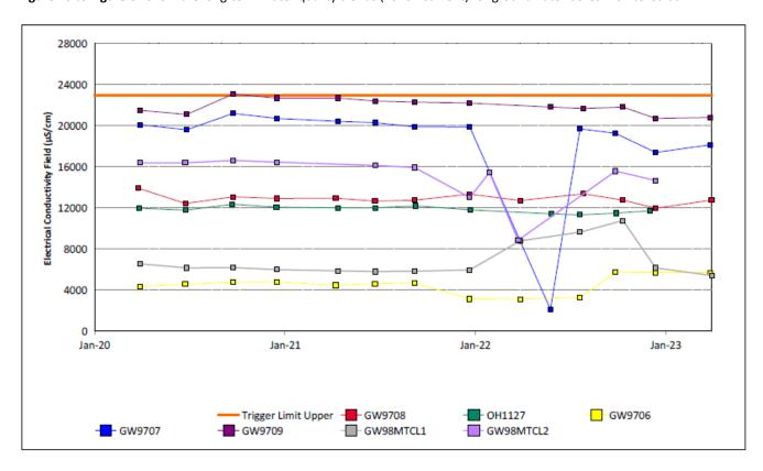
Figure 16: Bayswater Seam Electrical Conductivity Field Trend – March 2023
