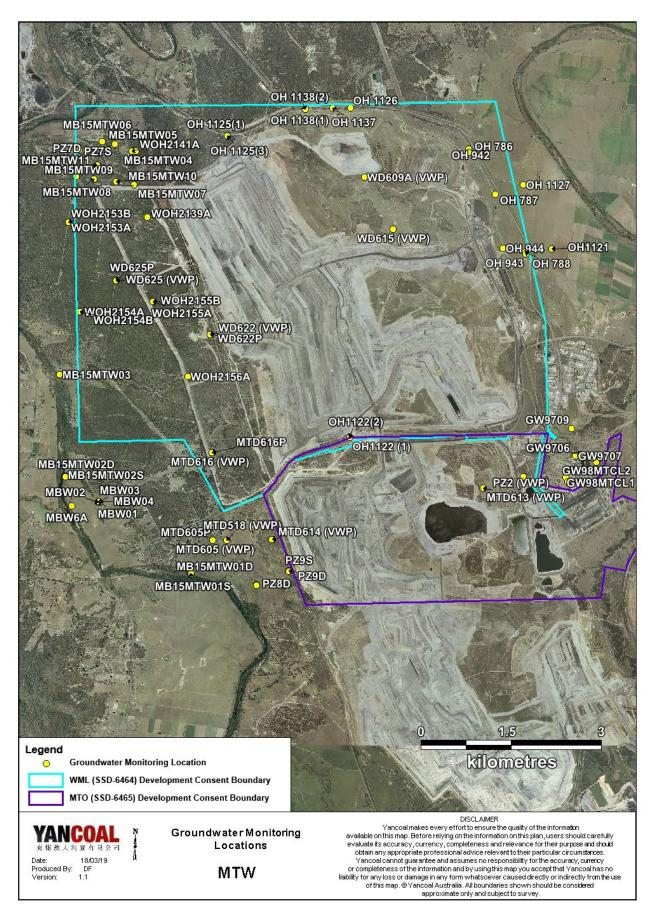
Figure 65: Groundwater Monitoring Location Plan
