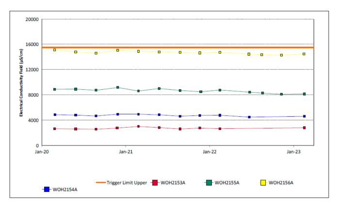
Figure 25: Redbank Seam Electrical Conductivity Field Trend – March 2023
