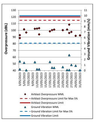
Figure 10: Bulga Village Blast Monitoring Results – May 2023
