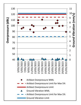
Figure 11: MTIE Blast Monitoring Results – May 2023
