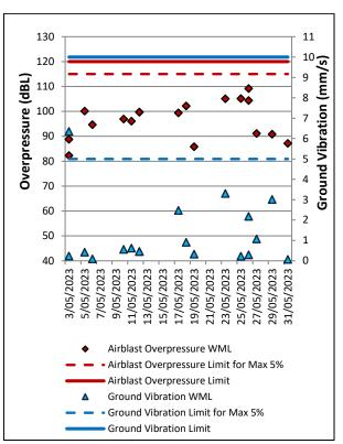
Figure 14: Warkworth Blast Monitoring Results - May 2023
