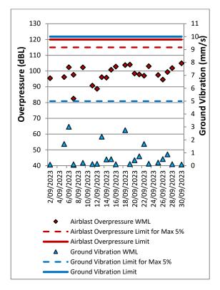
Figure 69: Wambo Road Blast Monitoring Results -September 2023
