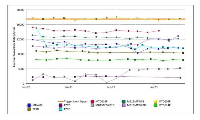
Figure 28: Shallow Overburden Electrical Conductivity Field Trend – September 2023
