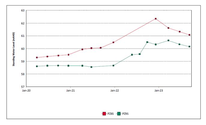
Figure 44: Wollombi Alluvium Standing Water Level Trend – September 2023
