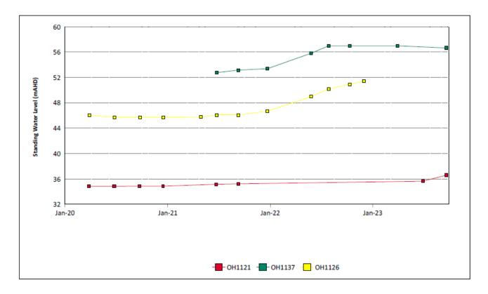
Figure 33: Vaux Seam Standing Water Level Trend – September 2023
