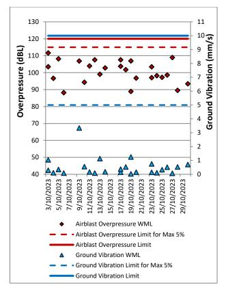
Figure 13: Wambo Road Blast Monitoring Results – October 2023
