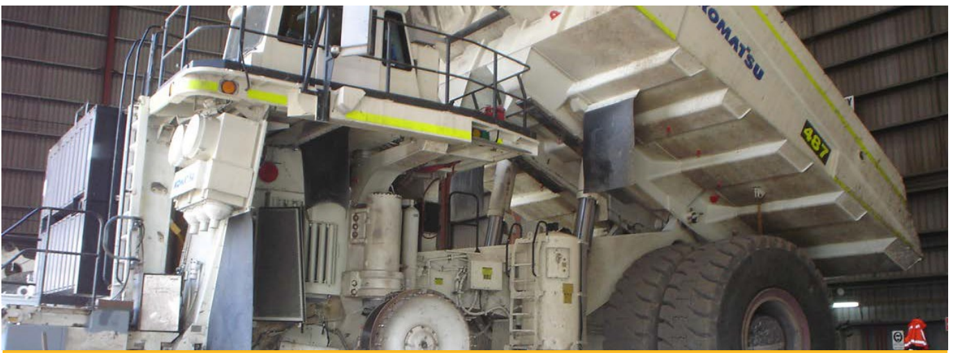
Haul truck being fitted with sound suppressing equipment
