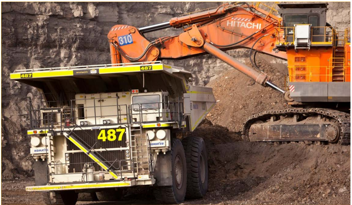
Minimising tip heights when loading and unloading helps to reduce dust across Hunter Valley Operations
