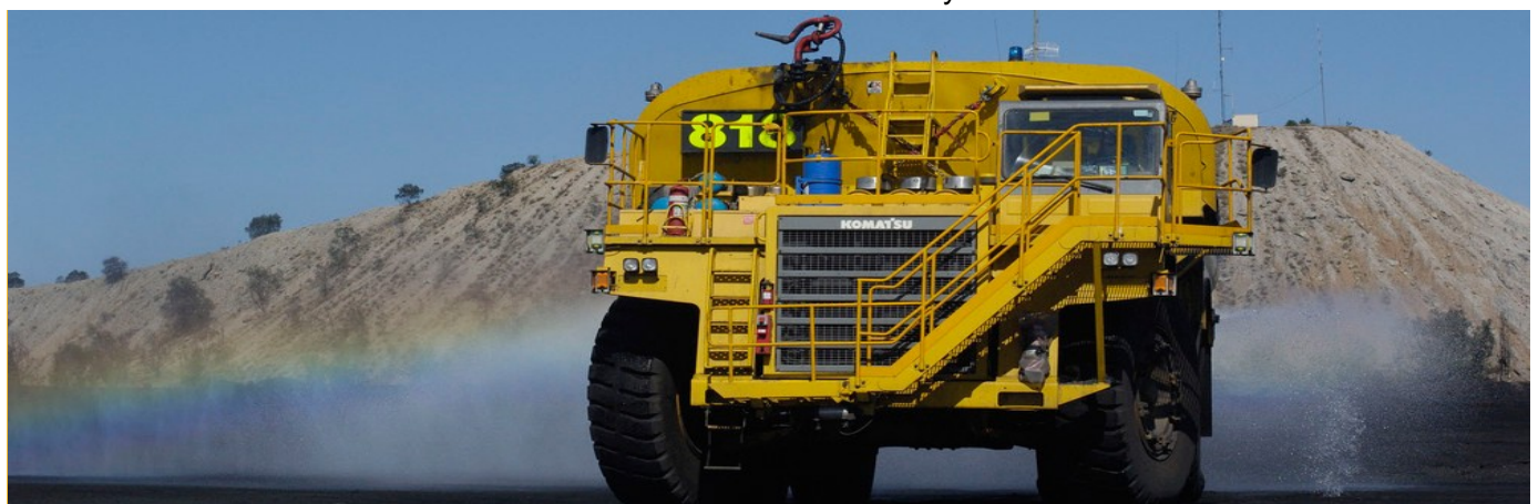
Water trucks continuously dampen haul roads with recycled water to minimize dust
