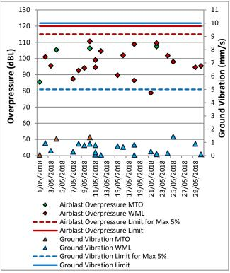
Figure 13: Wambo Road Blast Monitoring Results - May 2018
