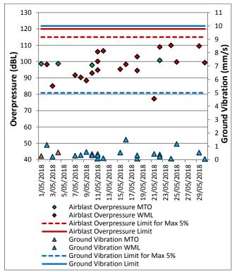
Figure 14: Warkworth Blast Monitoring Results – May 2018
