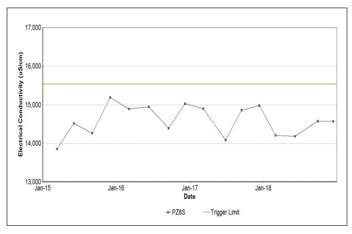
Figure 40: Wollombi Alluvium 1 Electrical Conductivity Trend – December 2018
