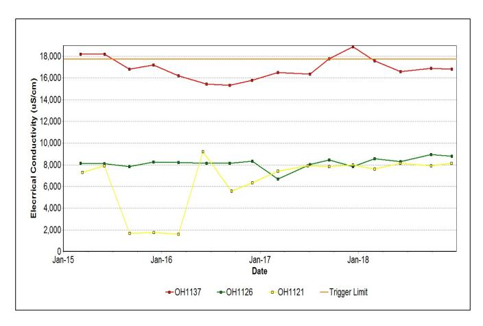
Figure 31: Vaux Seam Electrical Conductivity Trend – December 2018
