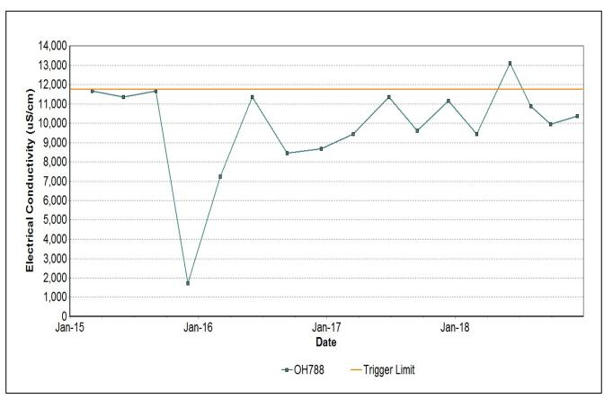
Figure 58: Hunter River Alluvium 6 Seam Electrical Conductivity – December 2018
