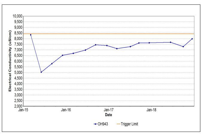
Figure 54: Hunter River Alluvium 4 Seam Electrical Conductivity Trend – December 2018
