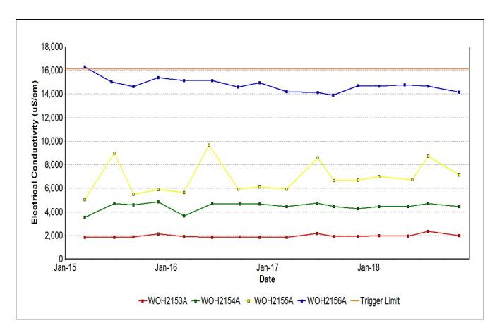
Figure 25: Redbank Seam Electrical Conductivity Trend – December 2018
