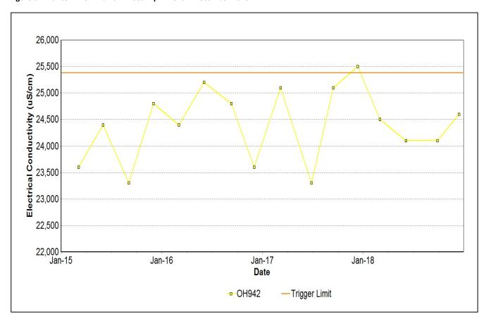
Figure 52: Hunter River Alluvium 3 Seam Electrical Conductivity Trend – December 2018
