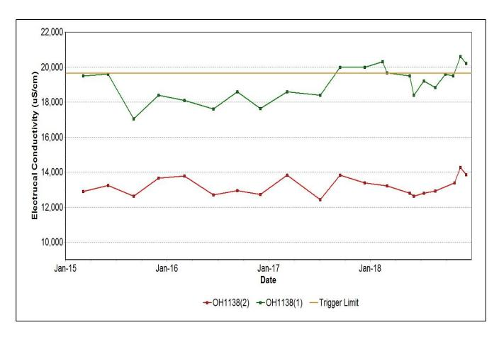
Figure 37: Warkworth Seam Electrical Conductivity Trend – December 2018
