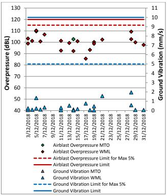
Figure 66: Wambo Road Blast Monitoring Results – December 2018
