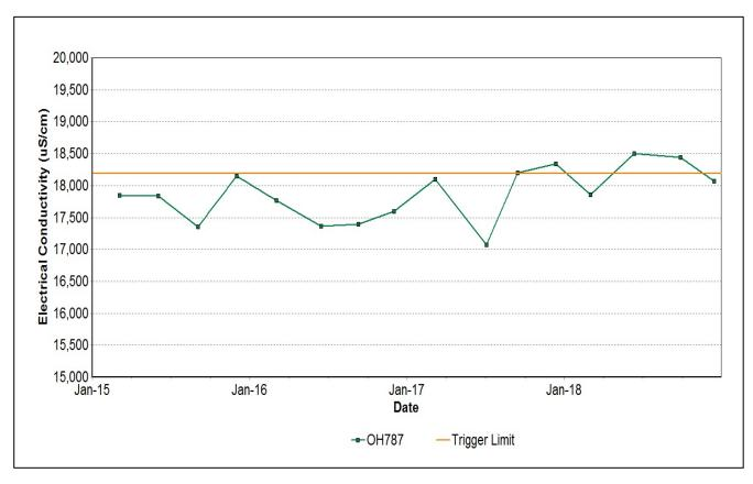
Figure 50: Hunter River Alluvium 2 Seam Electrical Conductivity Trend – December 2018
