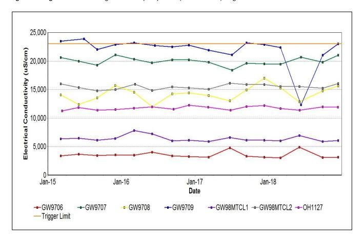
Figure 16: Bayswater Seam Electrical Conductivity Trend – December 2018
