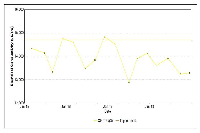
Figure 22: Bowfield Seam Electrical Conductivity Trend – December 2018
