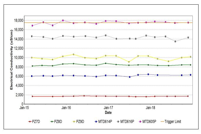
Figure 28: Shallow Overburden Seam Electrical Conductivity Trend – December 2018
