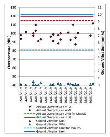
130 11 10 120 9 110 Ground Vibration (mm/s) 100 Overpressure (dBL 90 80 70 60 50 0 40 14/01/2019 20/01/2019 26/01/2019 28/01/2019 1/01/2019 8/01/2019 10/01/2019 12/01/2019 16/01/2019 18/01/2019 2/01/2019 24/01/2019 30/01/2019 5/01/2019 Airblast Overpressure MTO Airblast Overpressure WML Airblast Overpressure Limit for Max 5% Airblast Overpressure Limit **Ground Vibration MTO** Ground Vibration WML Ground Vibration Limit for Max 5% Ground Vibration Limit
