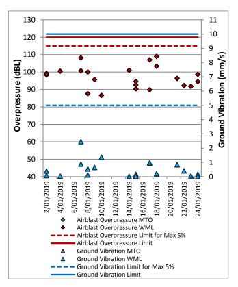
Figure 12: Wollemi Peak Road Blast Monitoring Results -January 2019
