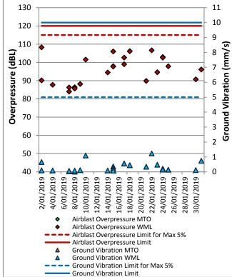
Figure 14: Warkworth Blast Monitoring Results – January 2019
