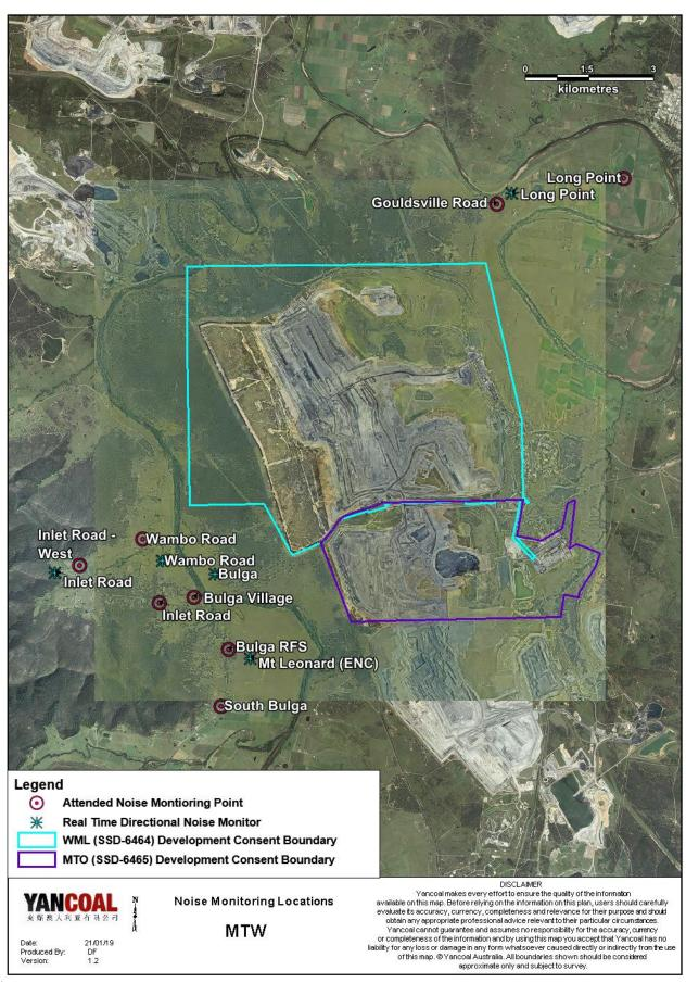
Figure 69: Noise Monitoring Location Plan
