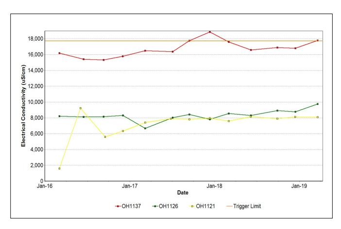
Figure 31: Vaux Seam Electrical Conductivity Trend – March 2019
