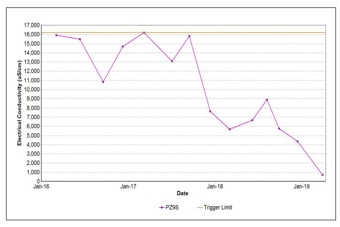
Figure 42: Wollombi Alluvium 2 Electrical Conductivity Trend – March 2019
