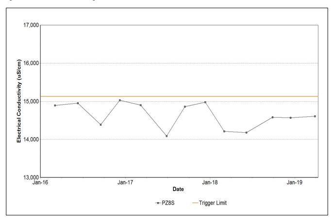
Figure 40: Wollombi Alluvium 1 Electrical Conductivity Trend – March 2019
