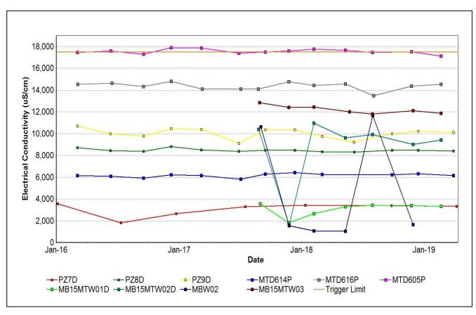
Figure 28: Shallow Overburden Seam Electrical Conductivity Trend – March 2019
