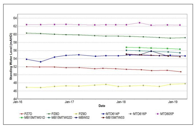
Figure 30: Shallow Overburden Seam Standing Water Level Trend – March 2019
