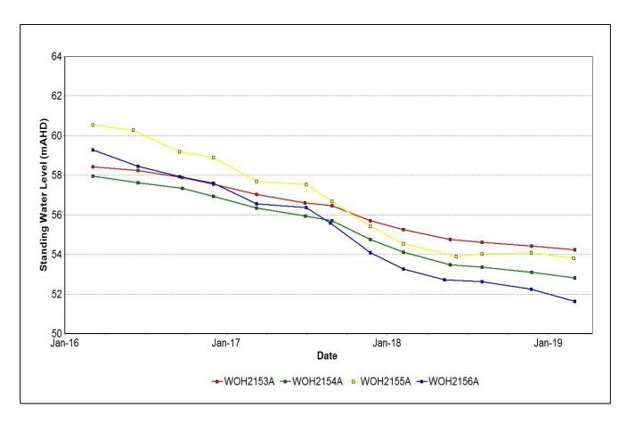
Figure 27: Redbank Seam Standing Water Level Trend – March 2019
