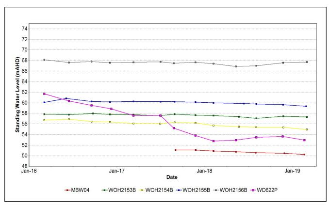
Figure 36: Wambo Seam Standing Water Level Trend – March 2019
