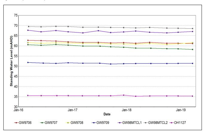
Figure 18: Bayswater Seam Standing Water Level Trend – March 2019
