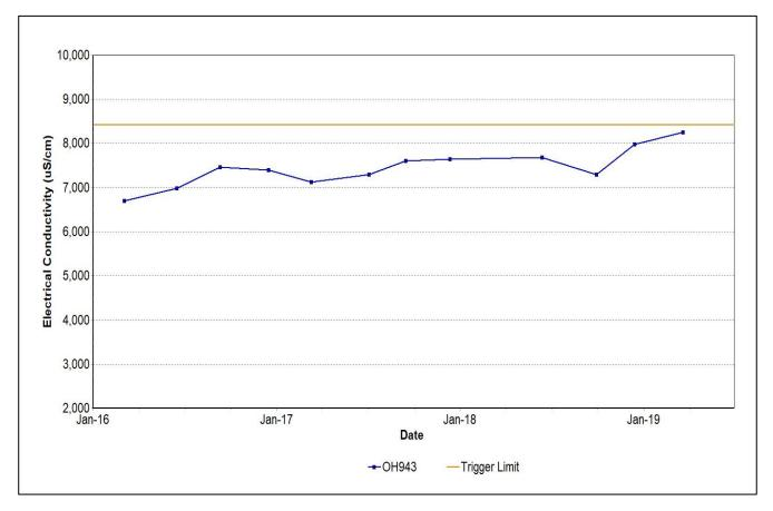
Figure 54: Hunter River Alluvium Electrical Conductivity Trend – June 2019
