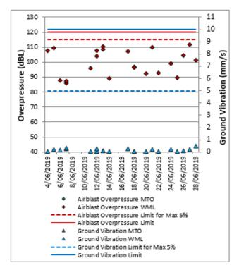
Figure 62: MTIE Blast Monitoring Results – June 2019
