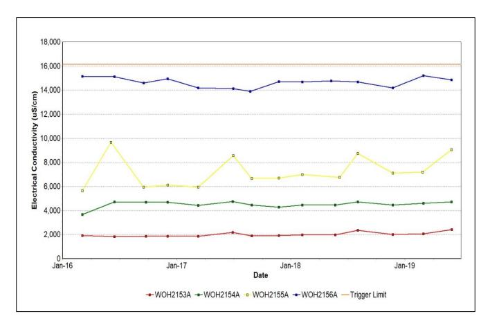
Figure 25: Redbank Seam Electrical Conductivity Trend – June 2019
