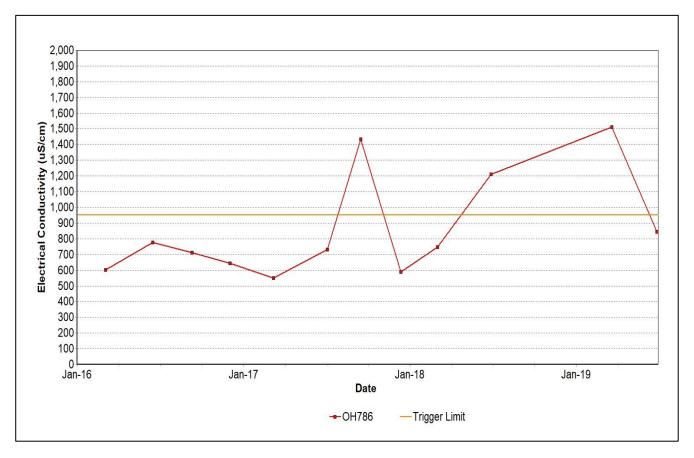
Figure 48: Hunter River Alluvium Electrical Conductivity Trend – June 2019
