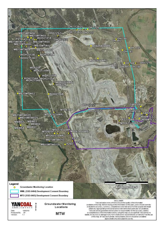
Figure 59: Groundwater Monitoring Location Plan
